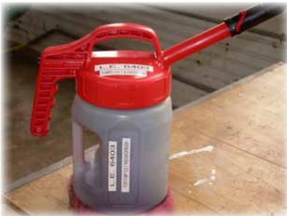
*This Oil Safe container holds Monolec 6403 for the DeLaval pumps. It is stored near the pumps.*
