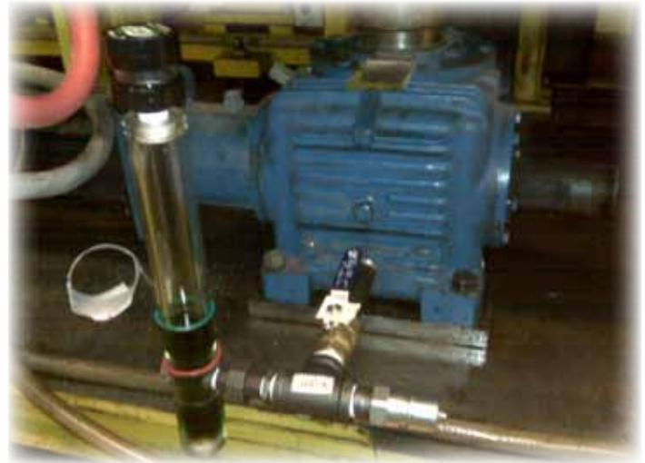
the gearbox drain ports to make oil drains easier. He suggested that the operator simply attach the hose from an existing filter cart to the AMS Quick Connect whenever the oil needed to be drained, then use the cart as a convenient transfer unit to get rid of the used oil.
