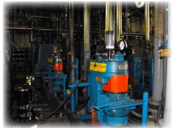
Desiccant breathers & online filtering with use of adapter kits
