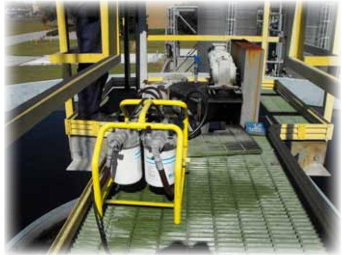
Online filtering of gear units
