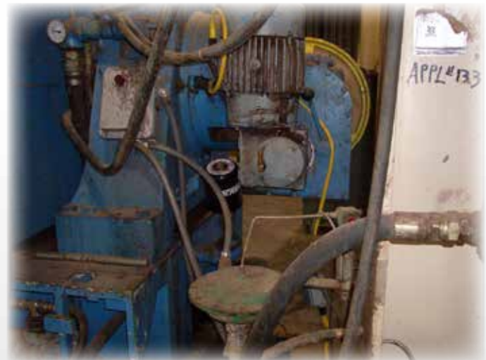
Photos before desiccant breather conversion. Above: no breather utilized. Below: pleated air filter only, no desiccant.
