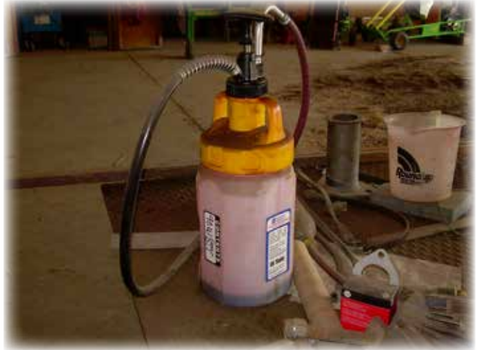
Oil Safe pump used to dispense LE Duolec 1605 (ISO 220).
