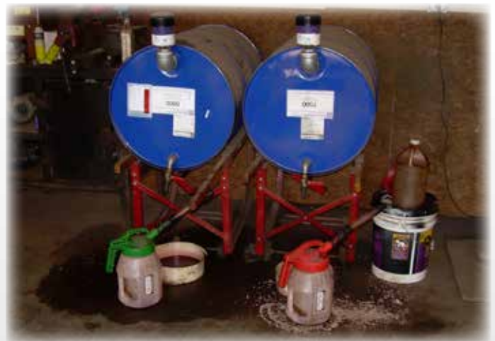
Des-Case breathers installed on two of the oil barrels and their corresponding Oil Safe containers. Notice the desiccant material is still dark blue when this picture was taken in early June 2008.
