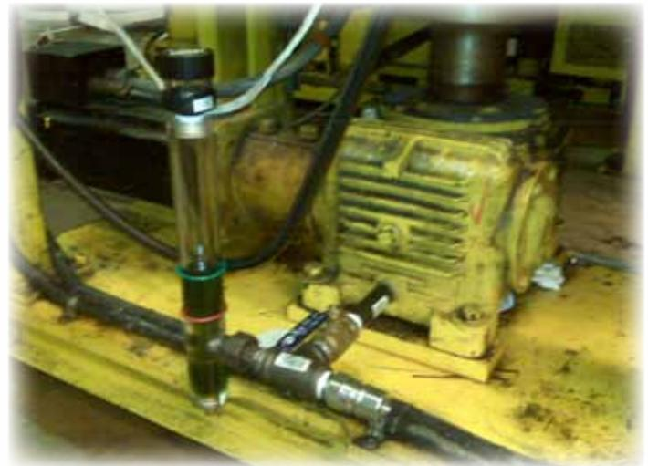
Mark recommended that all the gearboxes be flushed with LE's Monolec® R&O Compressor / Turbine Oil (6405) at no load, and then drained. After the flushing, he recommended the use of LE's Monolec Synthetic Industrial Lubricant (9460) in the cone drive.
