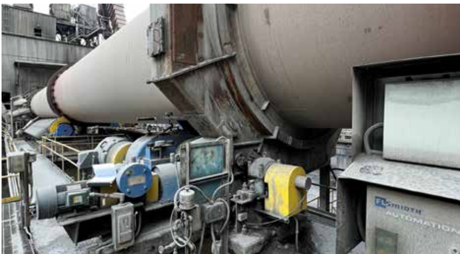
Prior to conversion, the lubricant buildup is significant.
