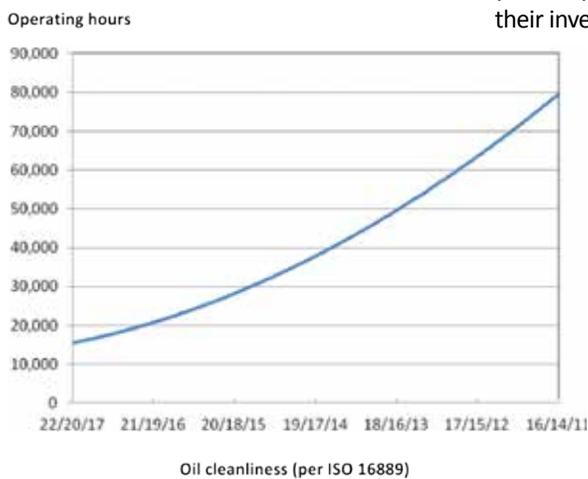
Figure 2: Projected engine life, with oil analysis.
