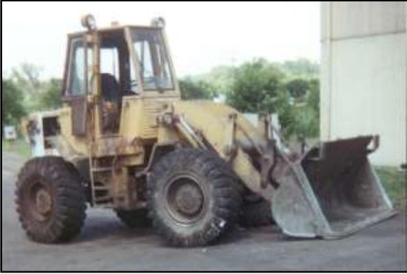
**This older CAT 920 front end loader gets limited use each year. LE's 8800 Monolec Ultra Engine Oil is only changed with planned maintenance at 300 hours.**
