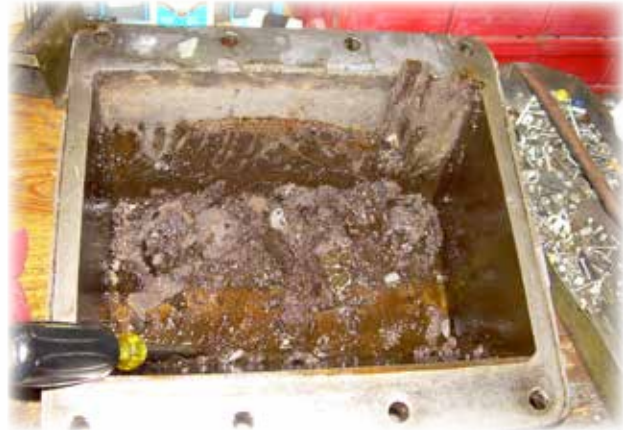
Valve body cover with sludge type deposit from using Shell Tellus product. Jim Robb reports no buildup from using LE 6403.
