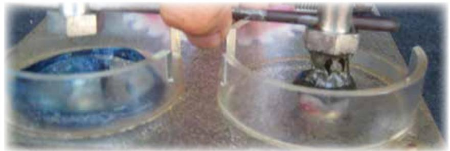
*Left: After the impact test, the previously used grease (blue) splashes, showing it is not suitable for the load. Right: Pyroshield 5182 grease remains at the hammer head, which means a film layer remains to protect against the friction caused by metal-to-metal contact.*
