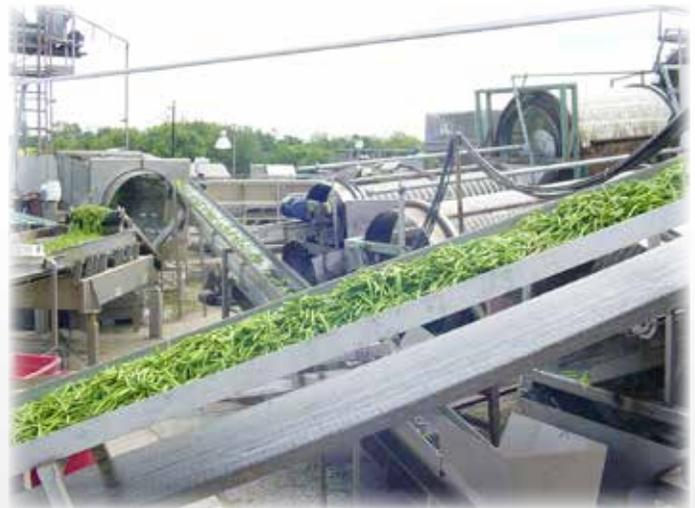
bean line in operation, it was obvious the grease they were using wasn't properly protecting their equipment. It was emulsified, running and oozing out of the bearings.
