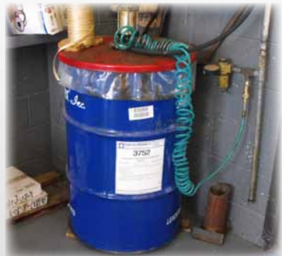
The shop uses Almagard Vari-Purpose Lubricant from an air-operated pump in a barrel.
