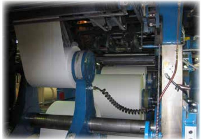
*CT50 Reel Tension Paster – handles 50 inch dia. rolls*
