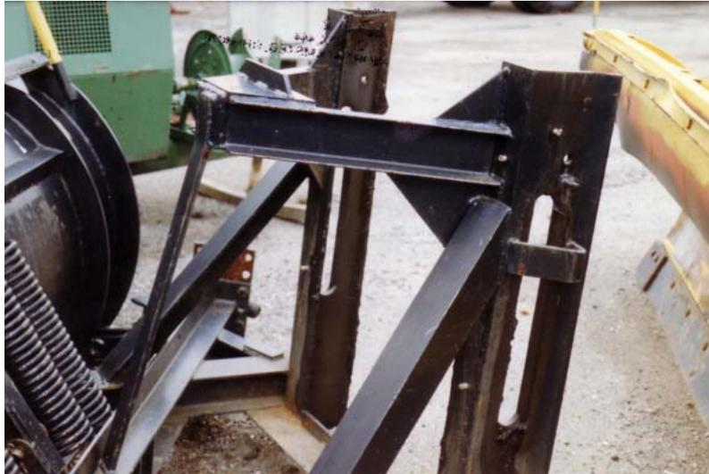
In the winter months, LE's 3752 is also used to lubricate the large frames on which the snowplows slide when they are raised and lowered. No other grease was able to withstand the adverse corrosive and washout effects of the salt and slush. LE's 3752 can handle the heavy loading of the plows. It stays in place and does not pound out, even under these severe conditions.
