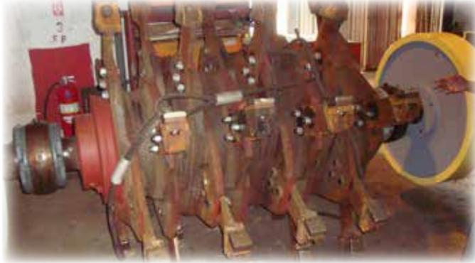
*The Unigrator rotating element removed for servicing*
