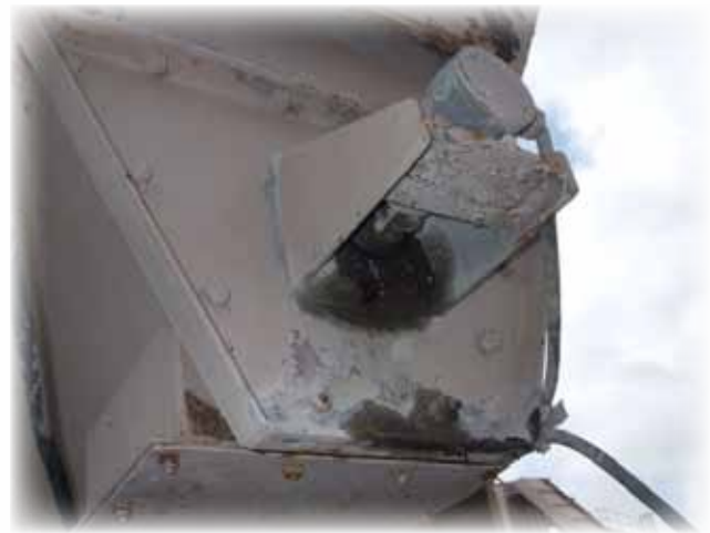
Spiral conveyor end shaft bearing using 3751.
