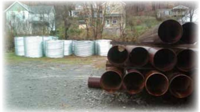
*Drill pad cellars and well conductor casings*
