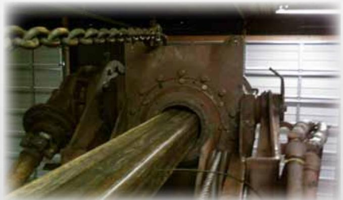
*Texoma 700 drilling rig main gearbox*
