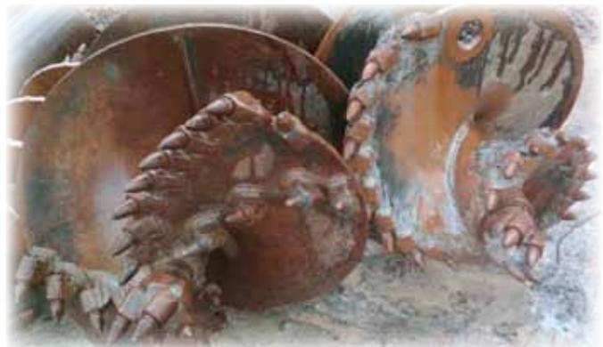
*Rock drill auger bits for drilling tough rock strata. Using bits like this, Ransom can drill holes from 12 to 36 inches in diameter.*
