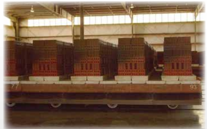
Kiln car with dried bricks waiting to be unloaded
