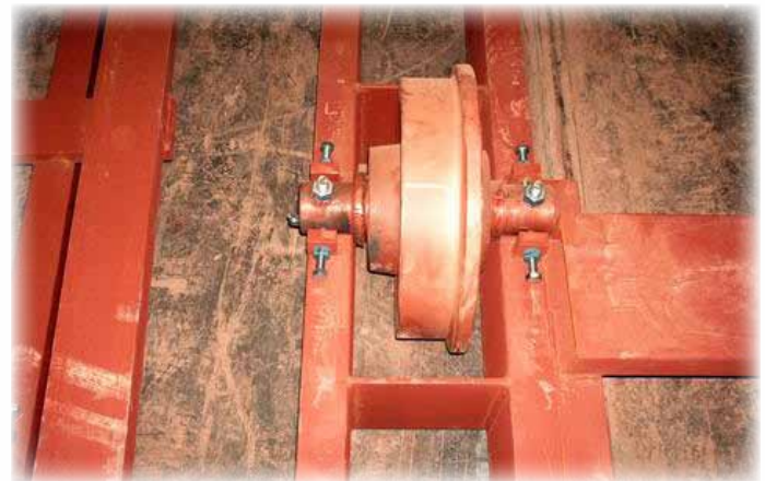
Kiln car wheels during assembly (above and below)
