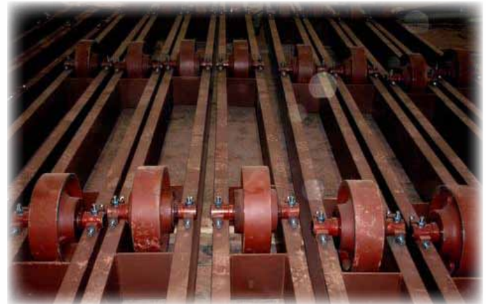
Kiln car wheels during assembly (above and below)
