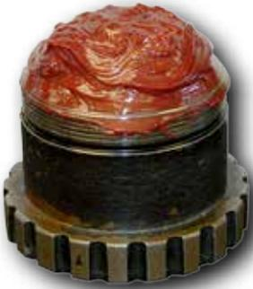
the tasks of hammering out hardened zerk fittings and chiseling old grease out of the bearings. To relube all of the cars, it took the lube technician 10 hours per day for eight days each month. At \$16 per hour, the labor dedicated to re-lubrication was costing approximately \$1,280 per month or \$15,360 per year.
