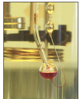
A viscometer is used in a laboratory to measure a hydraulic fluid's viscosity. (resistance to flow).
