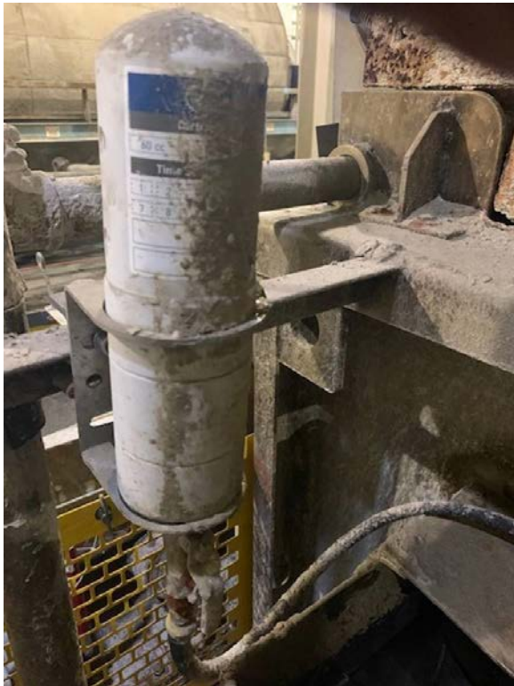
Single point lubricator (SPL) in use in a dirty environment.
