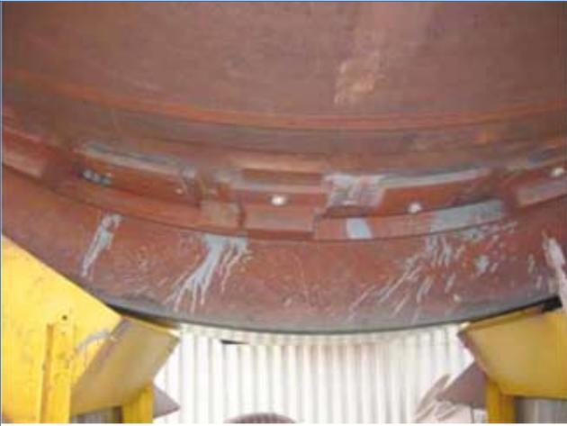
Figure 3. Wear pads in good condition.
