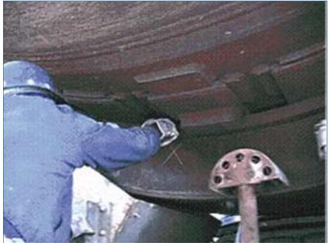
Figure 5. An operator inserts a lube bar between the tyre and the shell.
