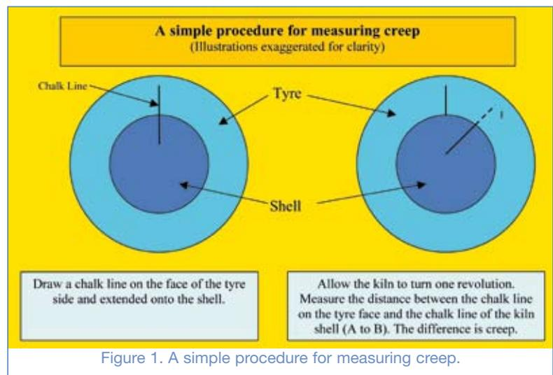
Figure 1. A simple procedure for measuring creep.
