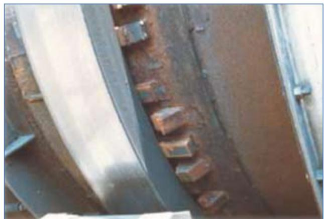
Figure 2. Wear pads in poor condition.
