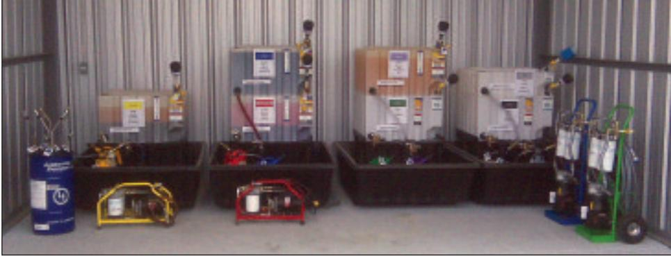
Stackable polypropylene tanks equipped with desiccant breathers, which can hold from 35 to 70 gallons of lubricants placed in large spillproof trays, are an example of safe and well-organized storage and is considered to be OSHA-compliant. The colored-framed units on the floor and the handheld carts are used for on-the-spot filtration of hydraulic oils or other lubricants. Photos courtesy of Lubrication Engineers, Inc.
