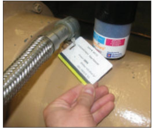
Color-coded tags can be placed at the lubrication points on the equipment to identify what proper lubricant is required.
