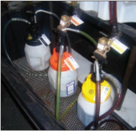
These are oil-safe, spillproof, OSHA-compliant containers equipped with hand pumps, five-foot hoses, and color coding. This type of container normally is used for filling small gear boxes.
