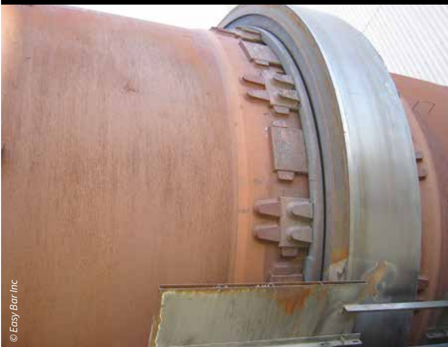
Placed between the tyre bore and shell, a solid lubricant bar will melt, coating the parts with a film of lubricant
