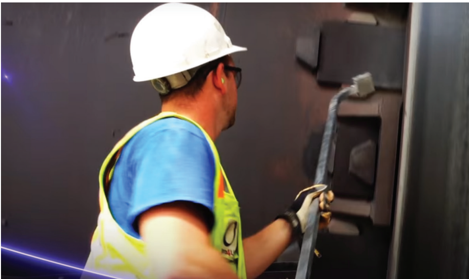
Easy Bar Lubricator 5-foot insertion tool is available for enhanced safety and faster application times
