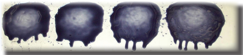
Spray pattern after converting to Pyroshield Syn Open Gear Lubricant. The spray nozzles do not clog with the Pyroshield fluid lubricant, allowing a more protective, uniform film of lubricant to be applied to the gears.
