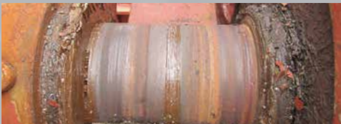
Anchor windlass lubricated with commercial grease – note the development of rust and wear as well as a lack of lubricant.
