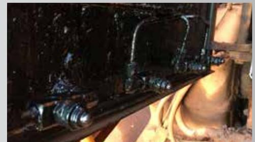
The spray nozzles on this open gear lubrication system remain clean and free of clogging while applying Pyroshield.
