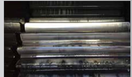
Clear, flowing Pyroshield 9011 is lubricating these ball mill open gears, making it easy for the operator to visually inspect with a strobe light during operation.
