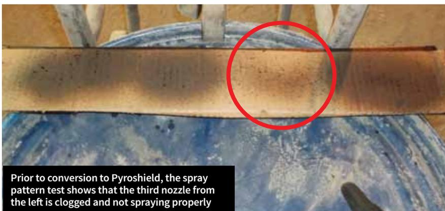
Prior to conversion to Pyroshield, the spray pattern test shows that the third nozzle from the left is clogged and not spraying properly
