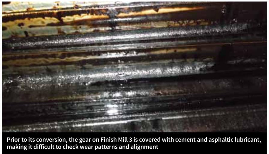
Prior to its conversion, the gear on Finish Mill 3 is covered with cement and asphaltic lubricant, making it difficult to check wear patterns and alignment
