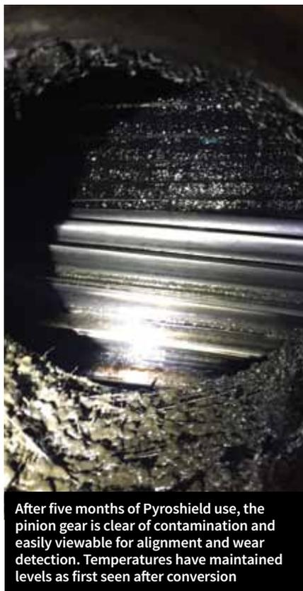
After five months of Pyroshield use, the pinion gear is clear of contamination and easily viewable for alignment and wear detection. Temperatures have maintained levels as first seen after conversion
