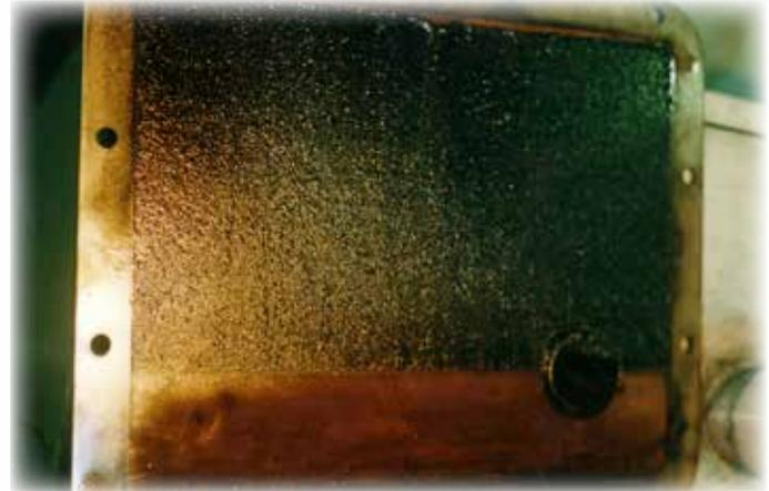
*After 30 days using Monolec 8420, deposits have been removed up to the oil level.*
