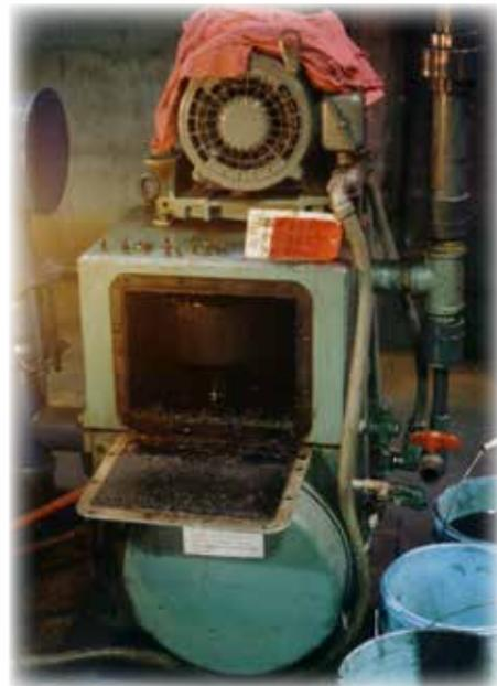
*Stokes vacuum pump model 212-11 with access with access cover removed. Note the plate is covered with carbon prior to converting to Monolec 8420.*
