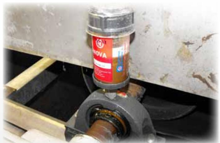
especially effective in severe operations caused by moisture or high temperatures. The lubricant's robust aluminum complex formulation seals out water and contamination and protects against oxidation, rust and corrosion. It also provides exceptional wear protection. Included in the formulation is Almasol, an LE proprietary additive which is a solid film additive that minimizes metal-to-metal contact further reducing heat, friction and wear.
