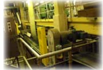
*Westside conveyor on right and incline conveyor (long flat and slanted line)*
