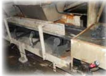
*Westside conveyor; product comes in from hopper above, notice Perma Nova unit on tail pulley.*
