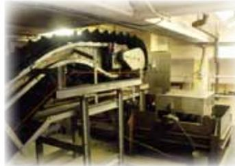
*Incline conveyor head pulley (upper), and reversing belt tail pulley (goes to incinerator). Perma Nova units are on each and Des-Case breather is on gearbox*
