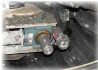
*Incline conveyor tail pulley (difficult access)*
