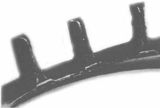
**Retainer failures** often lead to ring fracture or separation, followed by catastrophic failure, which may obscure the retainer that was the original problem. The most common cause of these failures in ball bearings is the flexing that takes place when the balls move in a criss-cross pattern because of misalignment. Retainer failures in other types of bearings are usually caused by handling damage, contamination, or marginal lubrication.
