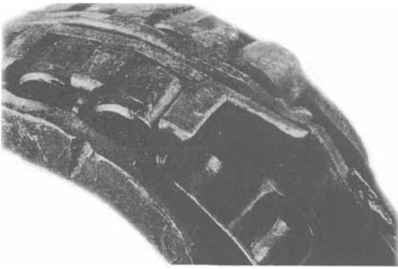
**Hot working** is a change in bearing geometry accomplished by a combination of heat and load. It is usually associated with complete or catastrophic failure. In some cases, the heat is generated within the bearing by lack of lubrication, friction from a ring turning on the shaft or in the housing, or excessive speed. In others, the heat enters the bearing from an external source, such as a heat-treating furnace. Sometimes two or more causes act together.
