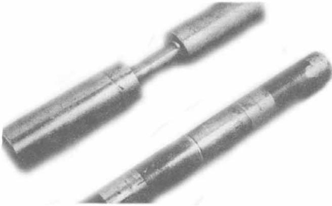
**Fretting** looks much like rust. It occurs in bores, on shafts and on other mating surfaces. It is caused by slight (even microscopic) movements under load. The wear particles are black if air has been excluded, red if it has not. Fretting can make the inner ring loosen on the shaft or “freeze” it so it cannot be removed; fretting can also cause the ring to break. It can be prevented by fitting parts too tightly to move under load; the manufacturer’s recommended tolerances should be followed.
