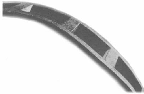
**Bending** is the permanent deformation of soft metal (not heat-treated) bearing components, such as retainers, seal carriers, flingers, and shields. In general, rings and rollers cannot be bent because the steel is too hard (see the photograph showing a broken inner ring.) In most instances, bending is caused by improper handling of the bearing or the part during installation or storage, but it may also be caused by an earlier failure of another type.
