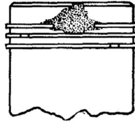
**Typical failure due to ring breakage.**
