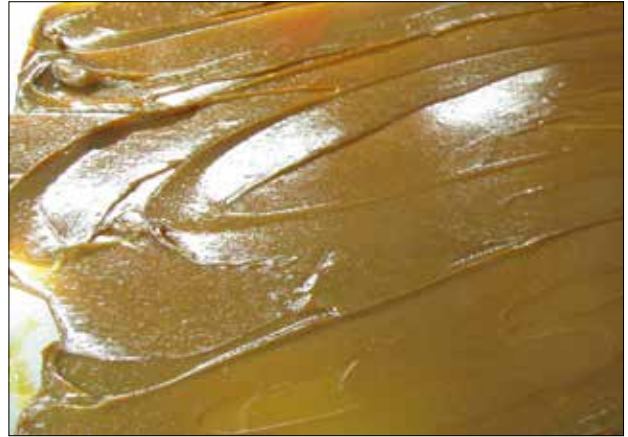
E. Initial testing of grease should include physical observation of color, odor, consistency and environment.
