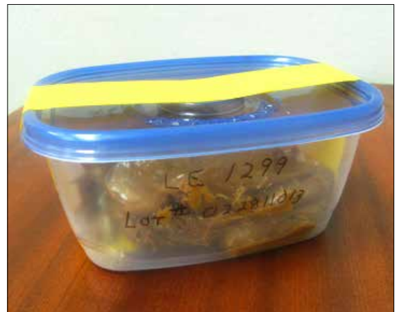
D. This disposable plastic container is an example of the proper way to ship a grease sample. It is sealed with tape and labeled with the product name and an identifying number for reference.
