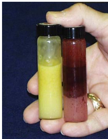
Sample on left shows water that has not separated from the oil. Sample on right shows water that is in process of separating from the oil.
