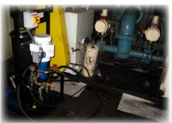
Stokes vacuum pump coupled with AMS filtration system
