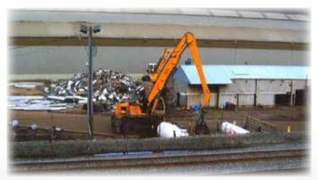
One of the model 934 Liebherr cranes used to sort scrap metals
