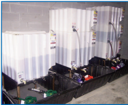
Tote-A-Lube poly tanks and Oil Safe containers in the lube room of FPL Foods, USA
