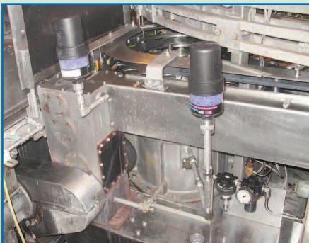
The Des Case Hydroguard breather is an ideal solution for management of lubricant condition in washdown applications.
